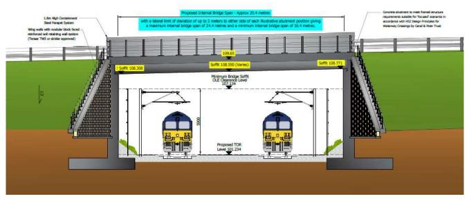
Note: extract taken from Proposed Document No. 2.18B "Proposed Bridge B1 Section and Elevation", (Drawing No. 1516-04250WDK-SI-C-301-006 Rev P14). Extract not to scale and provided for information purposes only.
