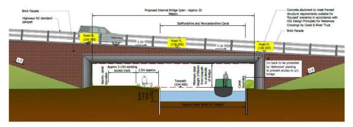
Note: extract taken from Certified Document No. 2.18D "Proposed Bridge B4 Section and Elevation", (Drawing No. 1516-04250WDK-SI-C-301-008 Rev P14). Extract not to scale and provided for information purposes only.
