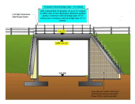
Note: extract taken from Proposed Document No. 2.18C "Proposed Bridge B2 and B3 Section and Elevation", (Drawing No. 1516-04250WDK-SI-C-300-007 Rev P14). Extract not to scale and provided for information purposes only.
