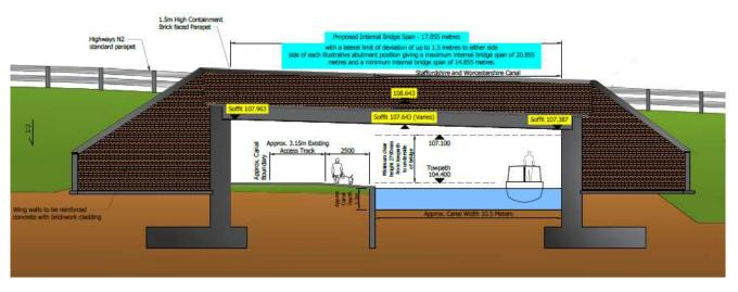
Note: extract taken from Proposed Document No. 2.18D "Proposed Bridge B4 Section and Elevation", (Drawing No. 1516-04250WDK-SI-C-301-008 Rev P17). Extract not to scale and provided for information purposes only.
