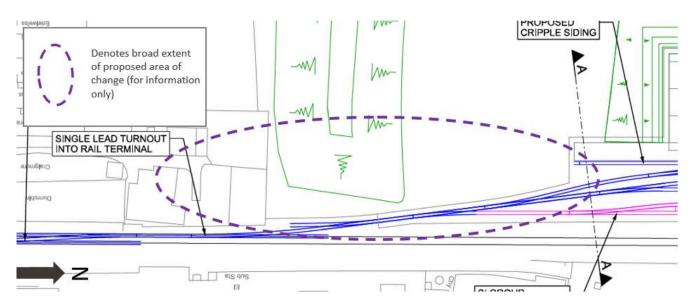
Note: extract taken from Certified Document No. 2.14 "The illustrative arrangement of railway alignment plan" (Drawing No. TRS-DRG-FA-001003 Rev 03). Extract not to scale and provided for information purposes only.
